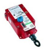
1CPS Series, Cable Pull Safety Switch, Cable, Maintained, 1NC/1NO Direct Opening, 1/2 NPT, Silver Contacts, 120 Vac LED
